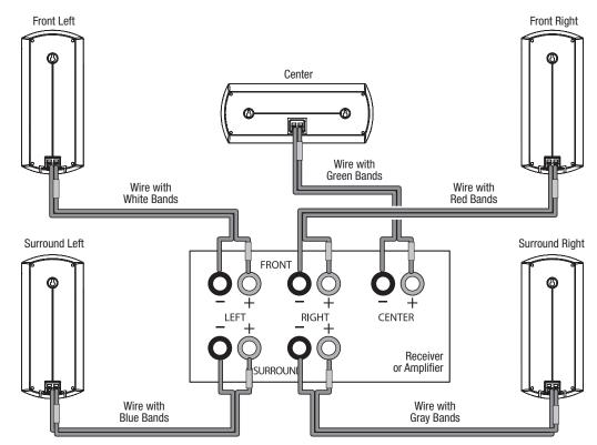
IMPORTANT: Make sure the ( + ) and ( – ) bare wires do not touch each other or the other terminal. Touching wires can cause a short circuit that can damage your receiver or amplifier.
