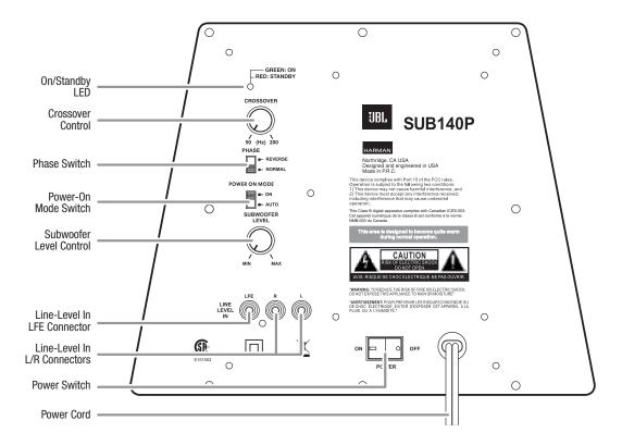
**On/Standby LED:** When the Power-On Mode Switch is in the "Auto" position, this LED indicates whether the subwoofer is in the On or Standby state:
