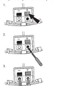
Connect the speaker's "+" terminal to the amplifier's "+" terminal:
