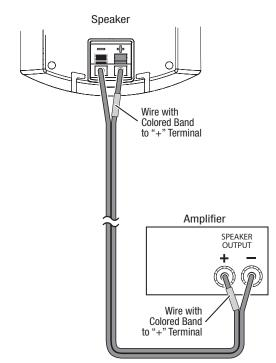
Connect the speakers to the proper amplifier channels:
